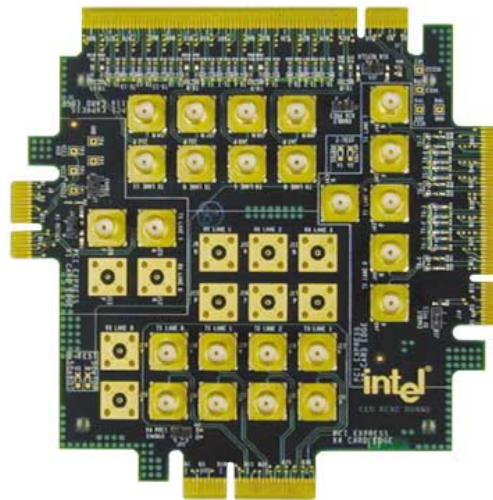
Figure 7. Compliance load board (CLB) for testing systems
