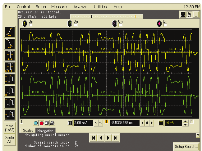
Figure 3. Lane-lane deskew and packet decode using E2688A SDA software with SigTest DLL
